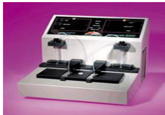
Fig 1.2.2.1 The FM-III Ferrograph, An Instrument In The Analytical Ferrograph System, Prepares Ferrograms For Analysis [1]
